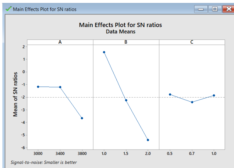
Fig. 3. Main effects plot for S/N ratio values of factors related to the surface roughness
