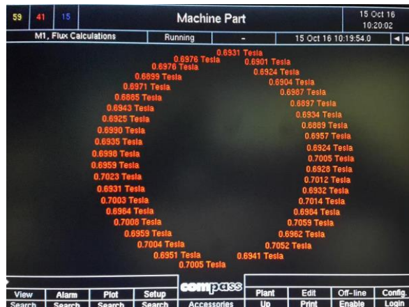
Fig.4. Distribution of magnetic flux on Hydro unit No. 1
