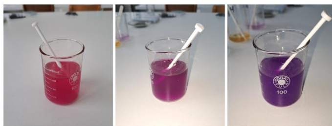
Fig. 6. Determination of calcium with the Palintest soil analyzer
