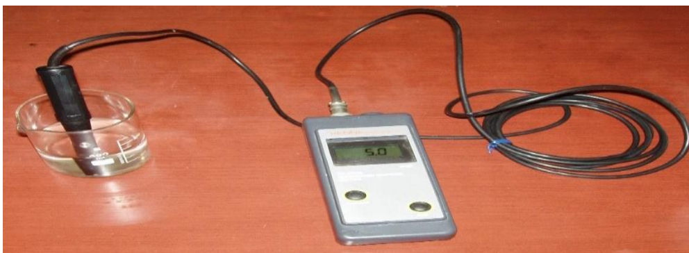
Fig. 3. Determination of oxygen content in small aliquot of aerated water using HANNA instrument with polarography sensor [1]
