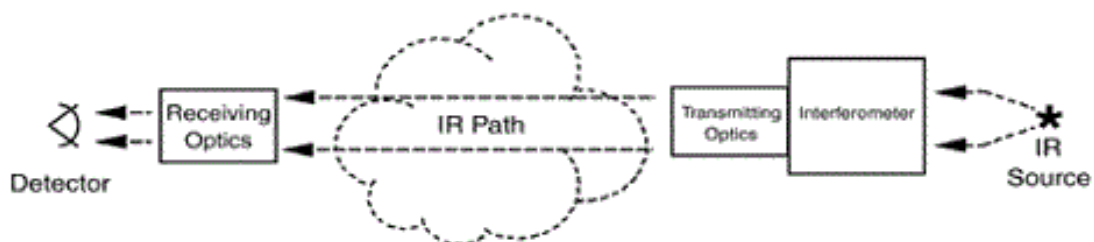
Fig. 2. Bistatic Configuration for Open-Path FTIR [5]
