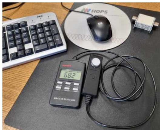
Fig. 16. Verification of model with lighting measurement
