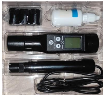
Fig. 3. BLE-9100 Device, Monitoring Dissolved Oxygen.
